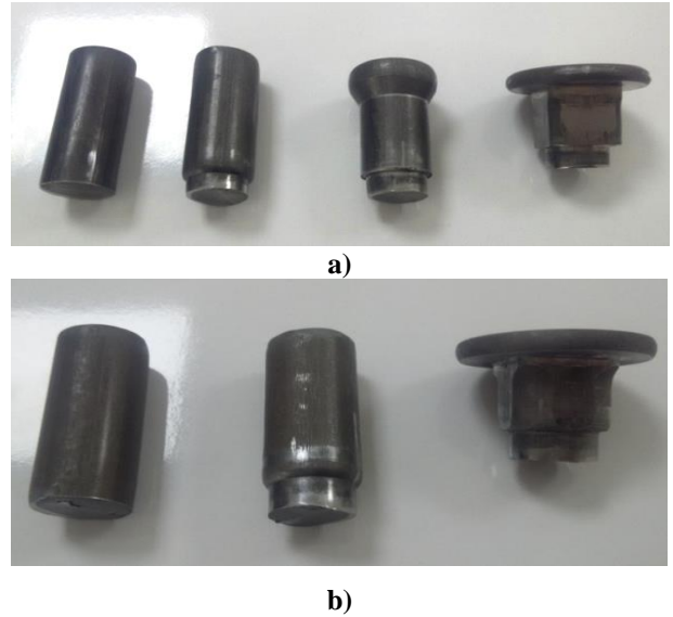
Figure 10. Prototype production of a) three-station and b) two-station design of sample.
